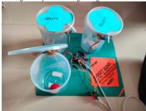
Figure 5: Automatically lid opening for bio degradable waste.
