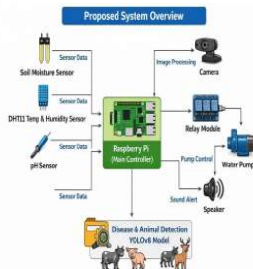
Figure 1: Proposed System Block Diagram
