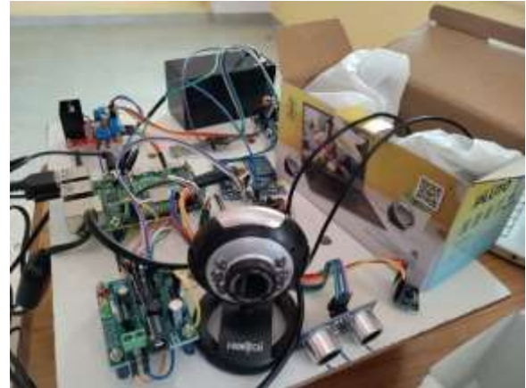
Figure 3: Experimental setup of the smart surveillance and sensor-based embedded system
