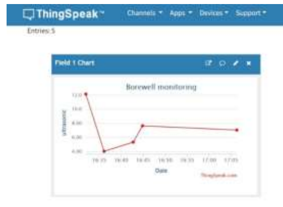
Fig. 4. HC-SR04 Ultrasonic Sensor Detection and Accuracy Results
