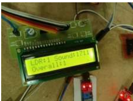
Fig3-Real-Time Sensor Data Display on LCD Module
